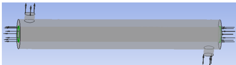
Figure 8. Setup boundaries for parallel fluid flow.
