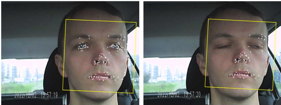
Figure 3a Feature points before blinking; b Loss of feature points after blinking.
