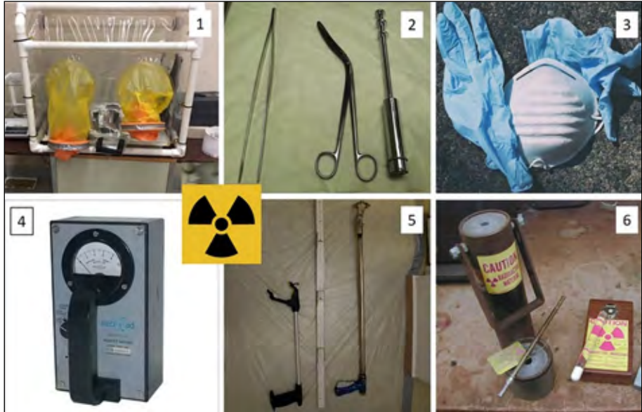
Fig. 2: Some objects at a crime scene which can indicate the presence of radioactivity (1. glove box; 2. tweezers; 3. gloves, masks; 4. radiation detectors; 5. manipulators; 6. radiation symbol and special shipping containers)
