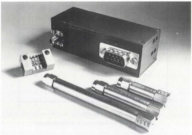
Fig. 8. Assembled six-port probe with microwave sub-assembly (left) and three of the calibration shorts (front)
