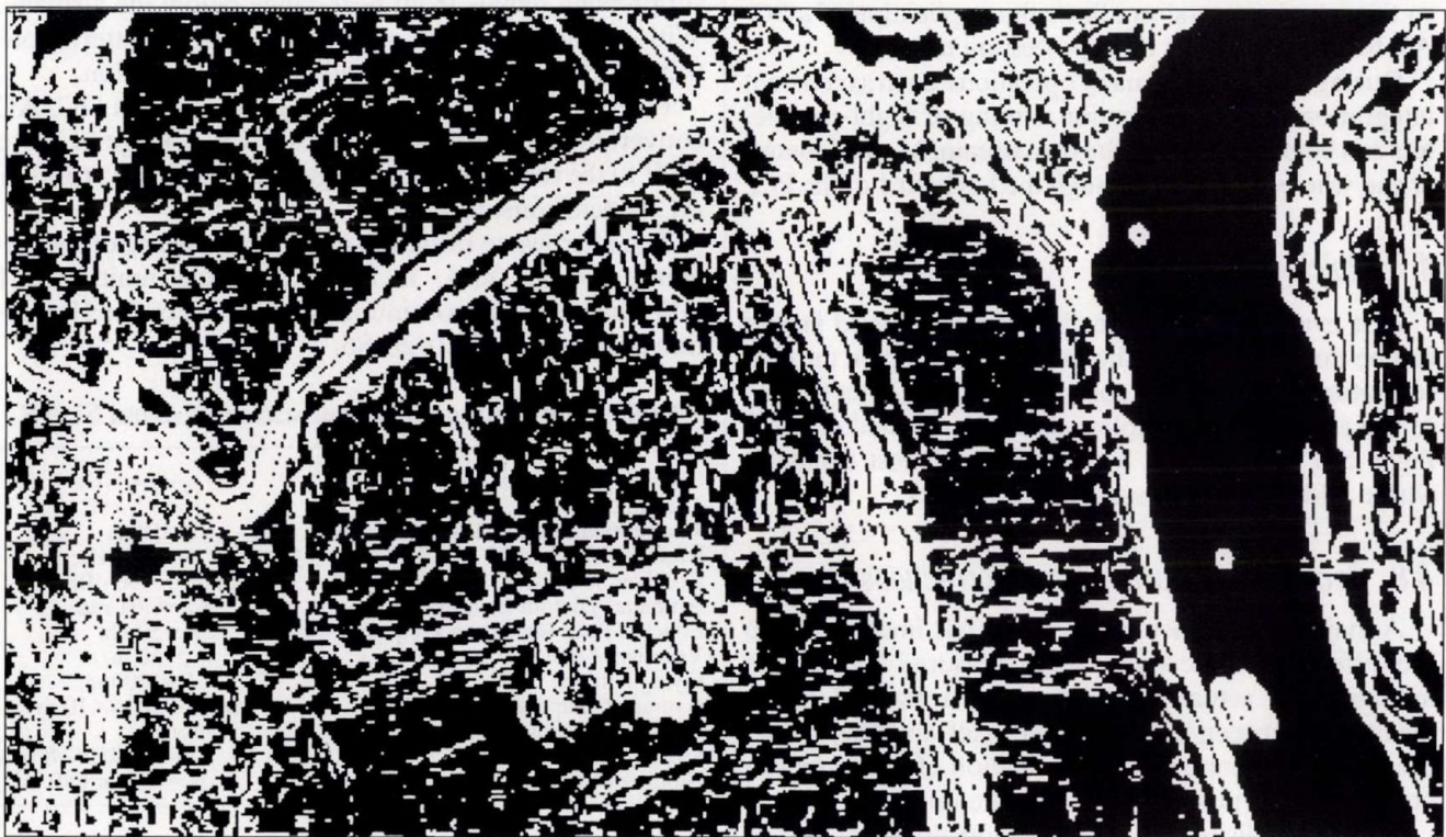
Fig. 6. The previous image after enhancing the edges
