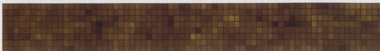
Fig. 31. Measured MC-variation of a PB of dimensions 2.07 x 16.5 m. The mean value of MC is 4% and the standard deviation is 0.48%.
