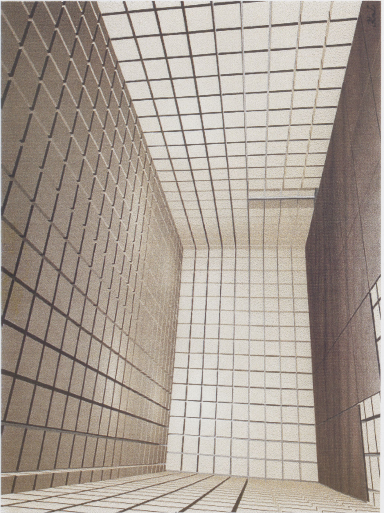
Fig. 5. Anechoic chamber using our absorbers (suggested for EMC tests in the 80-1000 MHz frequency band)
