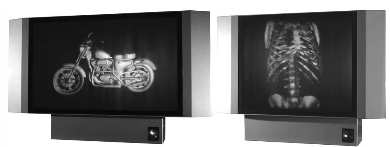
Figure 6. HoloVizio in operation – CAD and medical application
