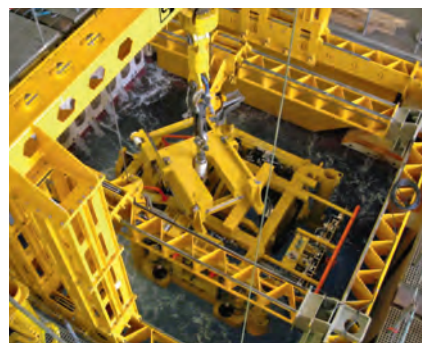
4. ábra. Module Handling System in Moonpool
